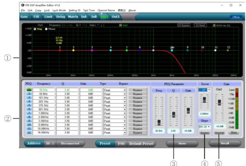
2. All parametric equalization parameters including gain, Q-factor, frequency and type are adjustable, with a bypass button available for selection, PEQ types include: Parametric EQ, Low Shelf, High Shelf, High-Pass-Filter, Low-Pass Filter, 180 Phase Shift, 360 Phase Shift.
