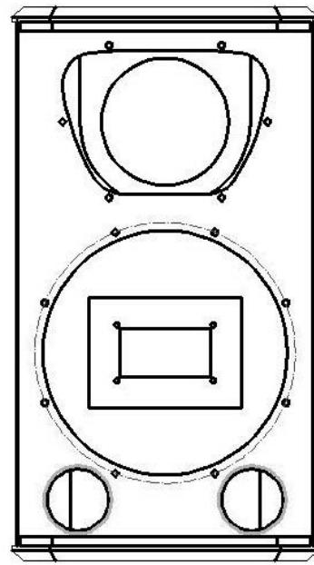
Equipped with one 10" speaker in a tuned enclosure. The HF section features one 1.5" compression driver from Celestion coupled to a diffuser, offering a dispersion of 90°x50° (H x V).
